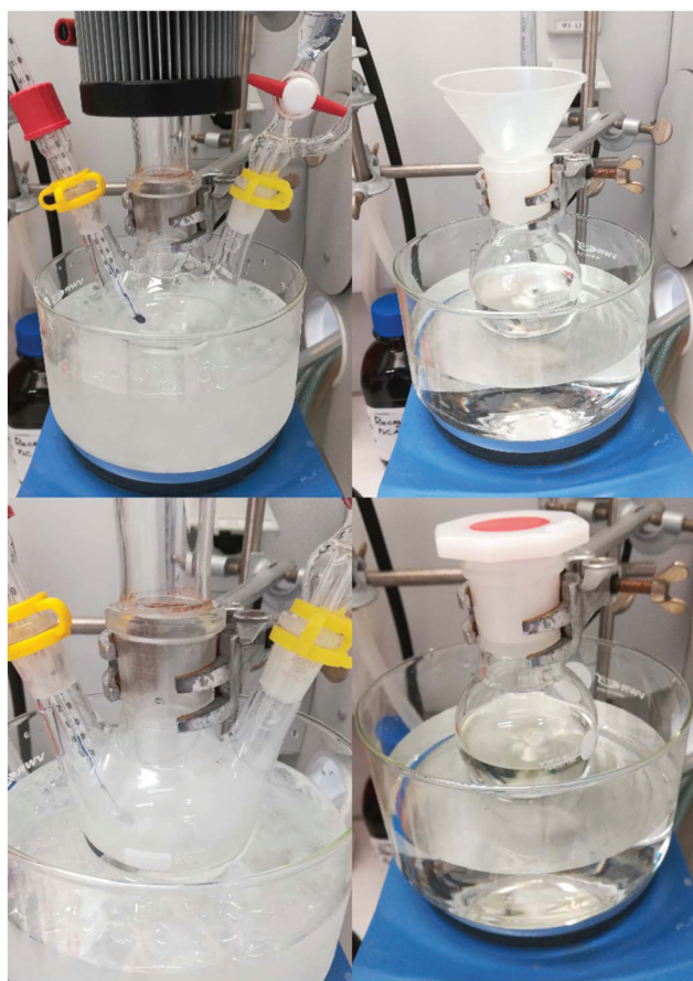
Fig. 2 Top left: dehydration of tert -butyl formamide (11.6 mmol in 35 mL DCM, 0.33 M), cooling is applied for subsequent addition of POCl 3 . Bottom left: reaction after addition of POCl 3 , internal temperature at 0 °C, still HCl vapors are evolving. Top right: dehydration of tert -butyl formamide (35 mmol in 35 mL DCM, 1.00 M), a water bath is applied for subsequent addition of p -TsCl. Bottom right: reaction after addition of p -TsCl. No visible hints of an exothermic reaction are observed. In some dehydrations, the temperature increased slightly.
