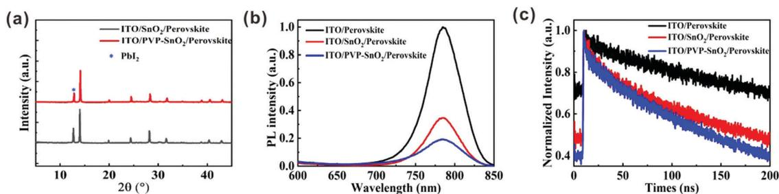
Fig. 4 (a) X-ray diffraction (XRD) patterns of the perovskites deposited on different ETLs. (b) Photoluminescence (PL) spectra of the perovskite films deposited on ITO, SnO<sub>2</sub> and PVP-SnO<sub>2</sub> substrates. (c) Normalized time-resolved photoluminescence (TRPL) spectra of the perovskite films deposited on ITO, SnO<sub>2</sub> and PVP-SnO<sub>2</sub> substrates.
