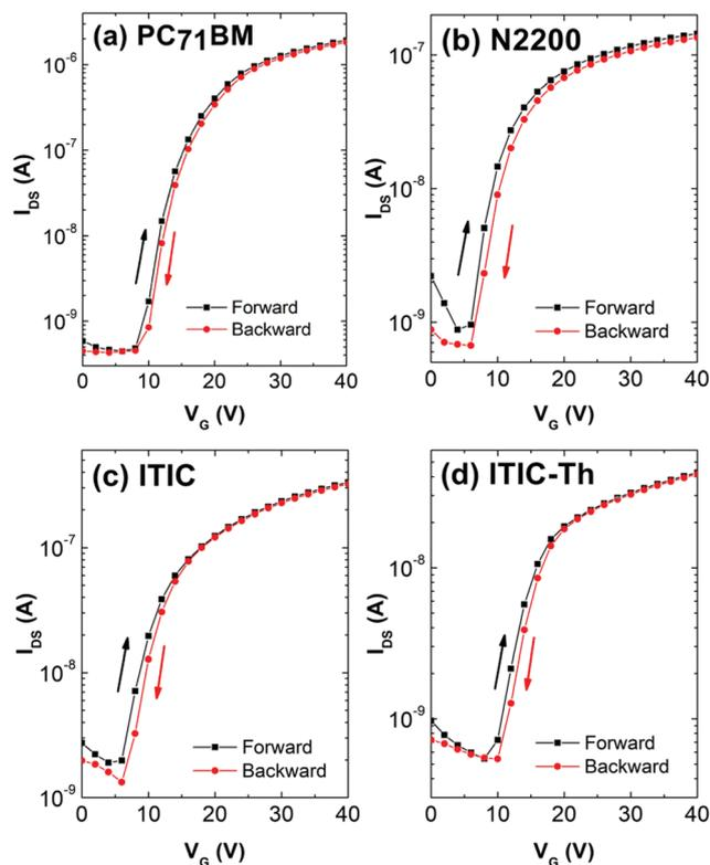
Fig. 5 Hysteresis study of (a) **PC<sub>71</sub>BM**, (b) **N2200**, (c) **ITIC** and (d) **ITIC-Th** with transfer characteristic at  $V_{DS} = 60$  V and  $V_G$  sweep rate of  $1$  V  $s^{-1}$ .
