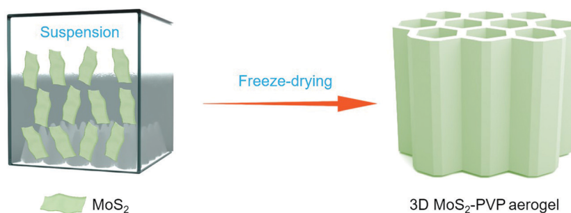
Fig. 1 Assembly process of the 3D MoS 2 -PVP aerogel.
