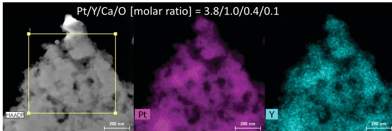
Fig. 3 Results of TEM-EDS for the reduced Pt<sub>2</sub>Y bulk nanopowder. The EDS spectrum is depicted as Fig. S6 (ESI<sup>†</sup>).
