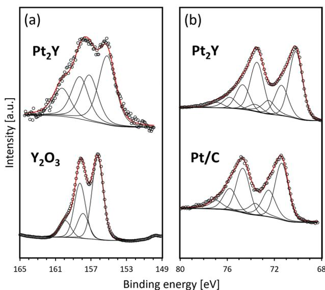
Fig. 4 XPS spectra of (a) Y 3d and (b) Pt 4f for the reduced Pt<sub>2</sub>Y bulk nanopowder and the references of Y<sub>2</sub>O<sub>3</sub> and Pt/C, respectively. Open circles are experimental data, and red lines are the fitting curves separated into some peaks.
