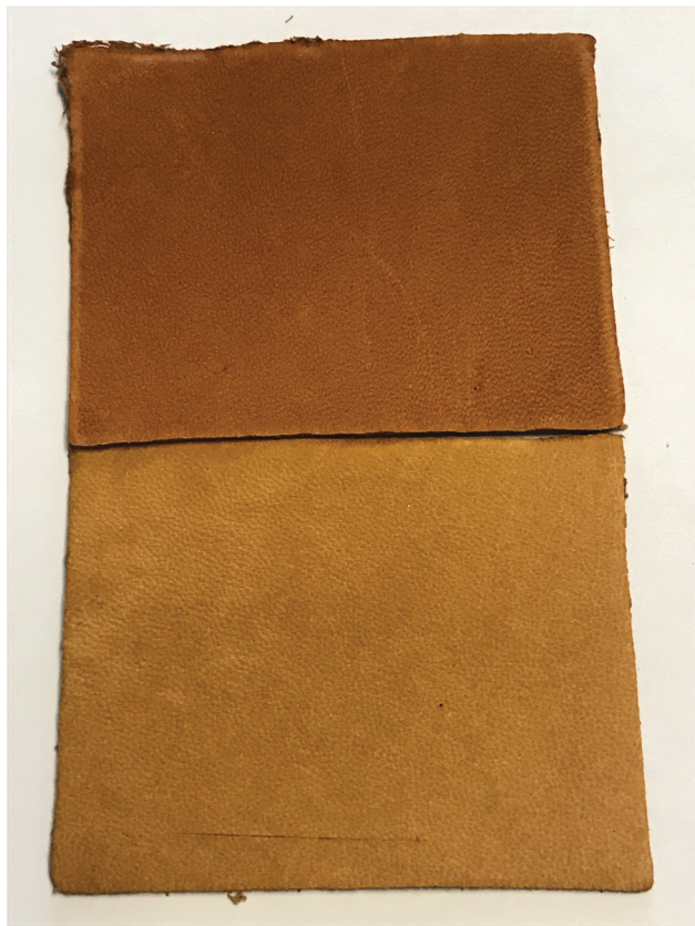
Fig. 4 Surface colour intensity for pieces retanned with PCE1000 (above) and AR (below).
