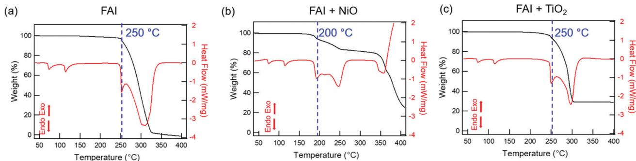
Fig. 1 TGA (black, left y-axis) and DSC (red, right y-axis) curves for (a) FAI, (b) FAI + NiO (1 : 1), and (c) FAI + TiO<sub>2</sub> (1 : 1) heated from 25 °C to 400 °C at 10 °C min<sup>-1</sup> under 100 sccm N<sub>2</sub> flow. The blue dashed lines represent the onset of thermal decomposition in each case.
