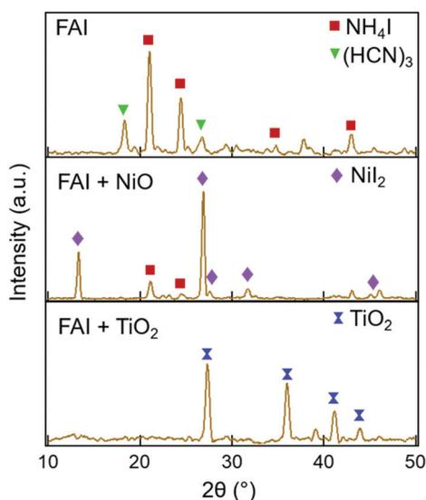
Fig. 3 XRD patterns of neat FAI (top panel), FAI + NiO (middle panel), and FAI + TiO<sub>2</sub> (bottom panel) after heating to 250 °C (brown) for 10 min. Peaks associated with crystalline NH<sub>4</sub>I, *sym*-triazine, NiI<sub>2</sub>, and TiO<sub>2</sub> are marked by maroon squares, green inverted triangles, violet diamonds, and blue dumbbells, respectively.
