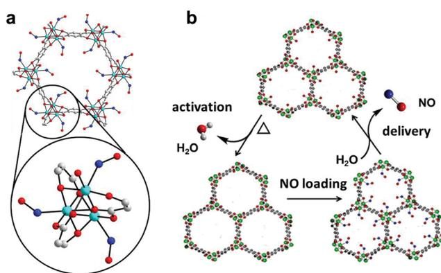
Fig. 1 NO adsorption and release by CPO-27 MOFs. Detail of the structural environment surrounding CUSs in CPO-27 MOFs with bound NO (refined from powder X-ray diffraction data): cyan – divalent metal ion (Co<sup>2+</sup> in this particular case), blue – nitrogen, red – oxygen, grey – carbon, hydrogen atoms have been removed for clarity (a); and schematic illustration of the NO-adsorption/release cycle (b).<sup>33</sup>
