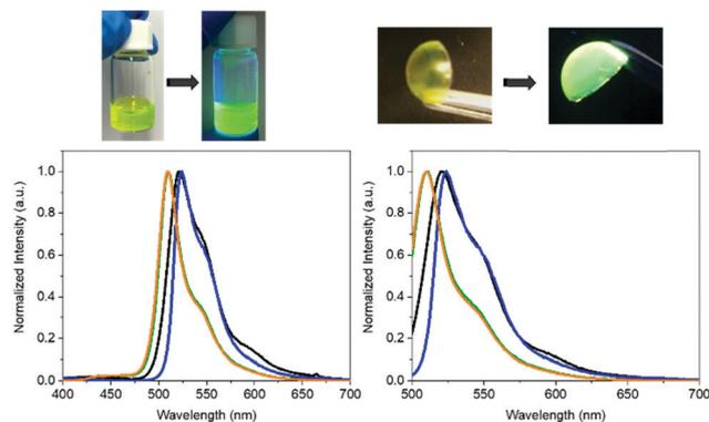
**Fig. 2** Top: Pictures of the FP-SF aqueous solutions (left) and films (right) under room and UV irradiation. Bottom: Emission spectra at excitation wavelengths of 375 nm (left) and 490 nm (right) of FP-SF aqueous solutions (green), FP aqueous solution (orange), FP-SF films (black), and FP-polymer films (blue).
