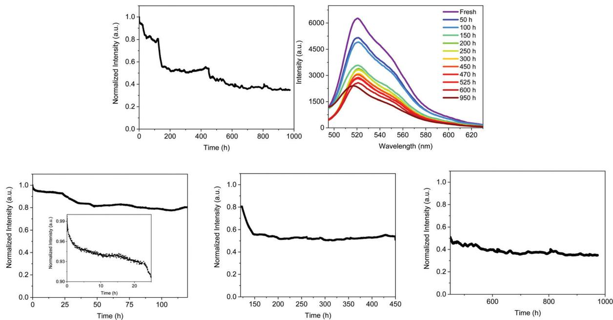
**Fig. 7** Typical performance of remote (2 cm) FP–SF based Bio–HLEDs operating at high applied currents at 200 mA. Top: Overall emission intensity decay (left) and the electroluminescence spectra changes (right) over time. Bottom: Emission intensity decay divided into four regimes, namely 0–24 h (inset graph), 24–120 h (left), 120–450 h (centre), and 450–1000 h (right).
