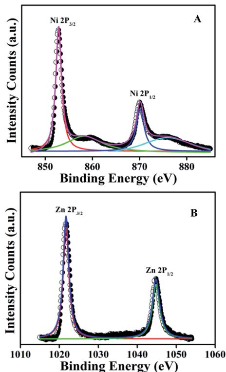
Fig. 2 High-resolution XPS spectra of the NiZn alloy, showing the (A) Ni 2p and (B) Zn 2p regions. The peaks indicate the presence of metallic Ni<sup>0</sup> and Zn<sup>0</sup> in the alloy.
