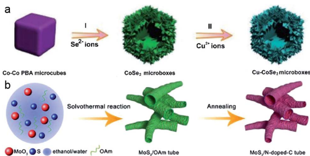
Fig. 14 (a) Schematic synthesis of Cu– \text{CoSe}_2 microboxes with two-step ion-exchange reactions. Reproduced from ref. 13, with permission from Wiley, 2018. (b) Schematic synthesis of \text{MoS}_2 /N-doped-C tube. Reproduced from ref. 50, with permission from Wiley, 2018.
