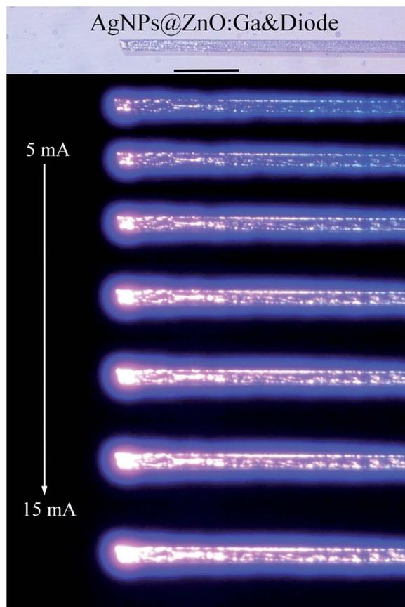
Fig. 2 The optical microscopy images of ultraviolet light emission from the n-AgNPs@ZnO:Ga MW/p-GaN heterojunction diode, with the injection current ranging from 5 to 15 mA (the scale bar: 100  $\mu\text{m}$ ).
