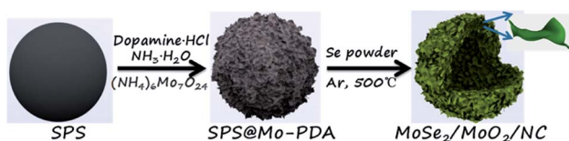
Fig. 1 Schematic illustration of the synthesis procedure of hollow microspherical \text{MoSe}_2/\text{MoO}_2/\text{carbon} ternary phases.
