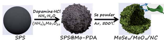
Fig. 1 Schematic illustration of the synthesis procedure of hollow microspherical MoSe 2 /MoO 2 /carbon ternary phases.
