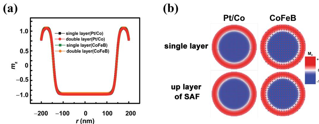
Fig. 2 Structure of a large skyrmion in a single FM circular plate and that in an SAF with no interlayer exchange coupling; (a) the  $M_z$  as a function of polar coordinate  $r$  and (b) the images of the skyrmion in the single layer and the upper layer of SAF.
