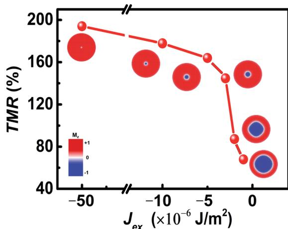
Fig. 7 Variations of resistance in the transition between a large skyrmion and a small one with change of  $J_{\text{ex}}$  for CoFeB ( $D = 2 \text{ mJ m}^{-2}$  and  $K_{\text{L}} = 1 \times 10^5 \text{ J m}^{-3}$ ).
