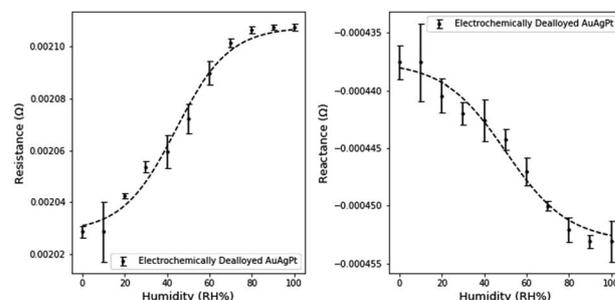
Fig. 9 Change in electrical characteristics with variations in humidity levels in electrochemically dealloyed NPG-Pt<sub>3</sub>.
