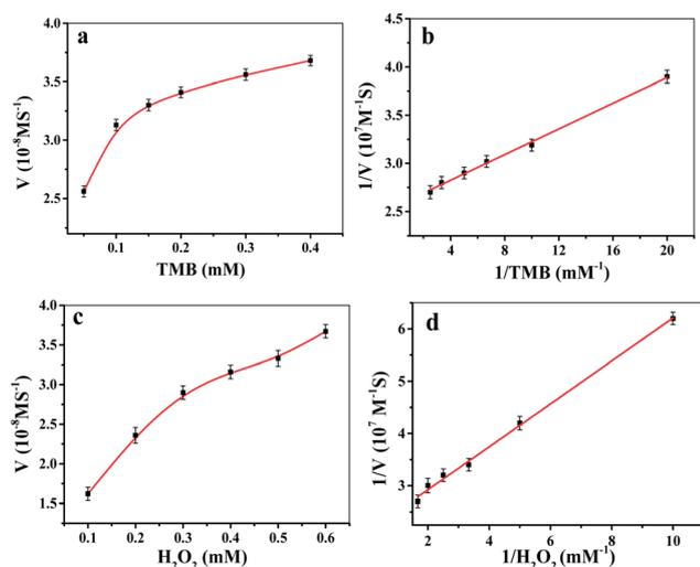
Fig. 3 Steady-state kinetic assay of the Fe-COFs composite by (a) changing the concentrations of TMB, and (b) changing the concentrations of  $\text{H}_2\text{O}_2$ , and the double-reciprocal model of the concentration of  $\text{H}_2\text{O}_2$  (c) and TMB (d).
