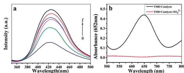
Fig. 2 (a) The fluorescence emission spectra of terephthalic acid in the presence of  $\text{H}_2\text{O}_2$  and different concentrations of Fe-COFs ((a-f)  $400, 500, 600, 700, 800,$  and  $900 \text{ } \mu\text{g mL}^{-1}$ ). (b) UV-vis absorption spectra of the peroxidase-like catalytic system with Fe-COFs in the absence and the presence of  $300 \text{ } \mu\text{M}$  sodium sulfite.
