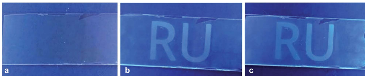
Fig. 6 Photographs of a thin PVP (55 kDa, 20% w/v in MeOH) film containing 1 (500 \mu\text{M} ) and 3 (10 mM) before (a), immediately (b) and 10 minutes (c) after exposure at 254 nm for 20 min through a RU-shaped 3D printed mask.
