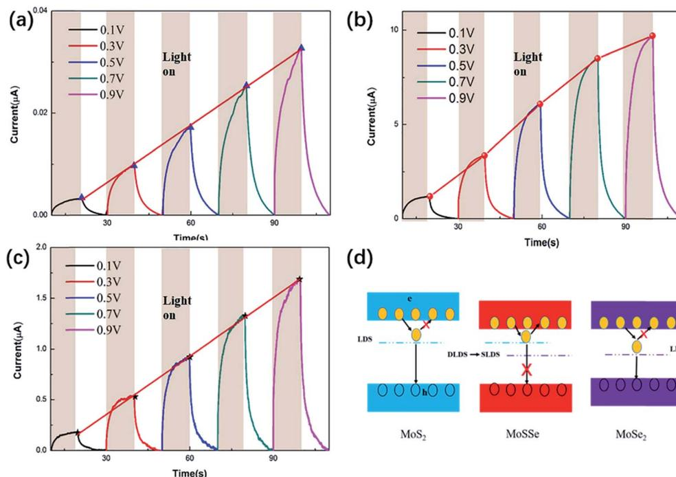
Fig. 5 The photocurrents of (a) MoS<sub>2</sub>, (b) MoSSe and (c) MoSe<sub>2</sub> at different bias voltages, and (d) schematic plot of the concept for suppressing DLDSs in MoSSe compared to MoS<sub>2</sub> and MoSe<sub>2</sub> by alloy engineering.
