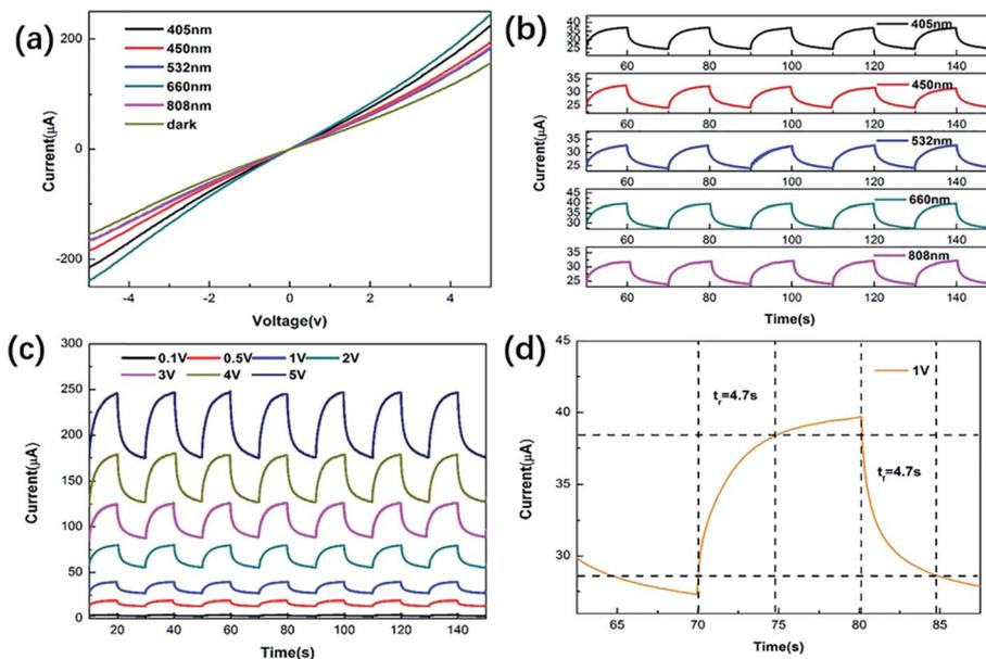
Fig. 3 Photoelectric characteristics of the MoSSe photodetector (a)  $I$ - $V$  curves at different wavelengths under dark conditions and at constant power ( $1.75 \text{ mW mm}^{-2}$ ), (b) the time-dependent photoresponse under irradiation with various lasers of  $1.75 \text{ mW mm}^{-2}$  at 1 V bias, (c) time-dependent photoresponse at different voltages, and (d) rise and fall times at a 1 V potential.
