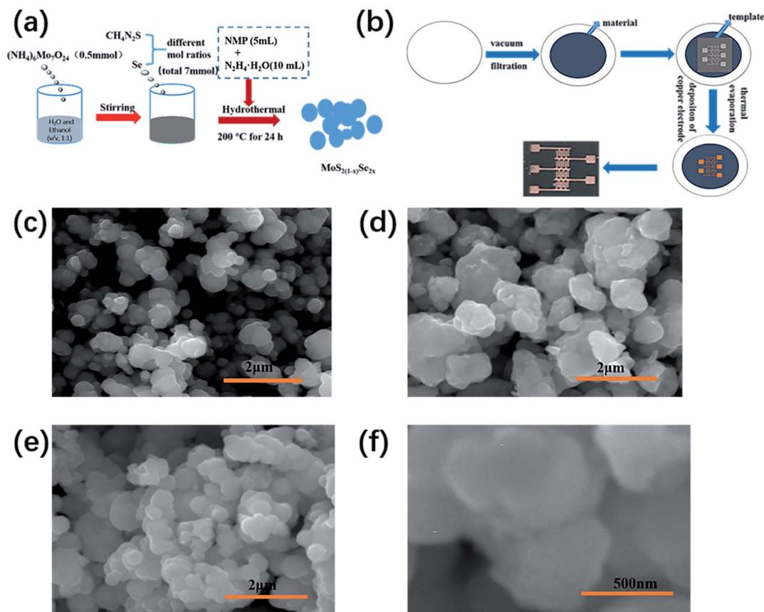
Fig. 1 (a) Schematic diagram of  $\text{MoS}_{2(1-x)}\text{Se}_{2x}$  synthesis, (b) schematic diagram of device preparation, and SEM images of (c)  $\text{MoS}_2$ , (d)  $\text{MoSe}_2$  and (e and f)  $\text{MoSSe}$ .
