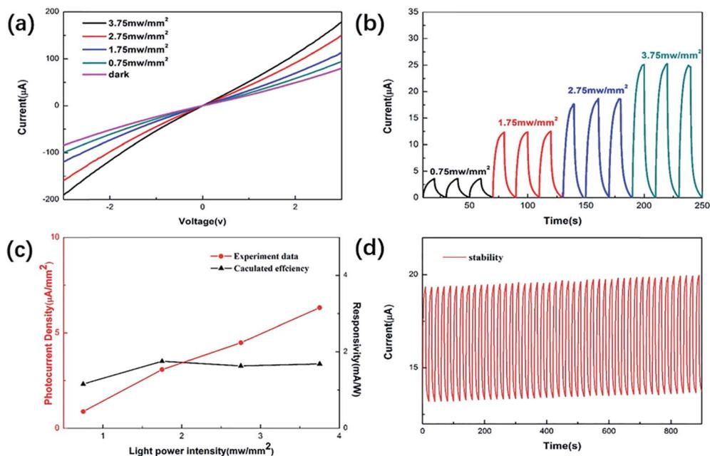
Fig. 4 (a) The  $I$ - $V$  curves of MoSSe samples under dark conditions and at different power densities, (b) photocurrent of the device at various power densities, (c) calculated photoconversion efficiencies of the device at various power densities, and (d) cycling stability measurements of the device.
