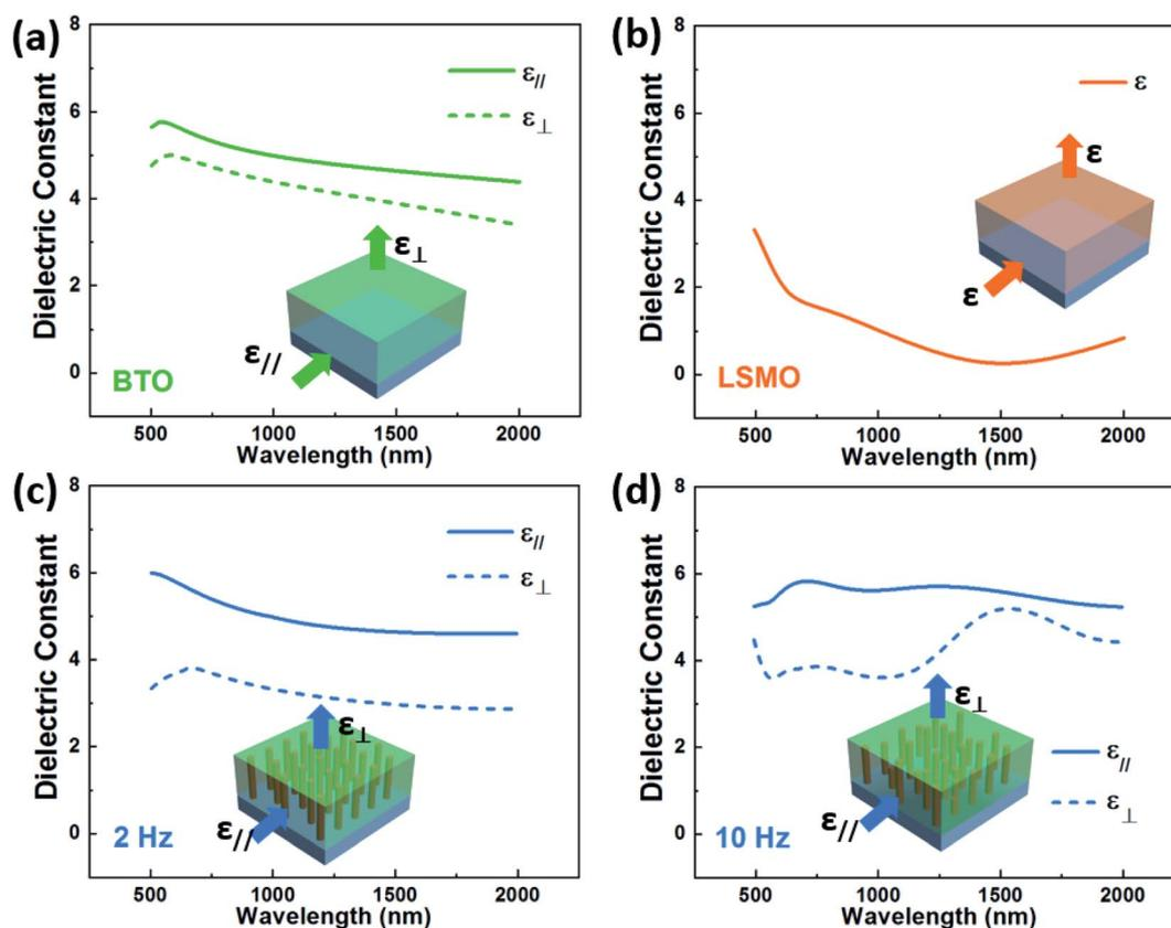
Fig. 4 Fitted real part of the dielectric constants for (a) pure BTO (b) pure LSMO (c) 2 Hz BTO : LSMO and (d) 10 Hz BTO : LSMO thin films. The ordinary and extraordinary curves are plotted in solid and dashed lines, respectively. The fitting direction of the dielectric constants is demonstrated in the inserted schematic drawings.
