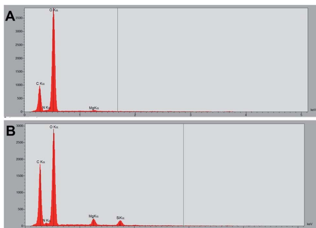
Fig. 9 Energy dispersive spectroscopy carried out on the surface of a tomato leaf. (A) untreated (reference) region. (B) treated region on which a drop of TO was deposited and immediately observed at the electron microscope.
