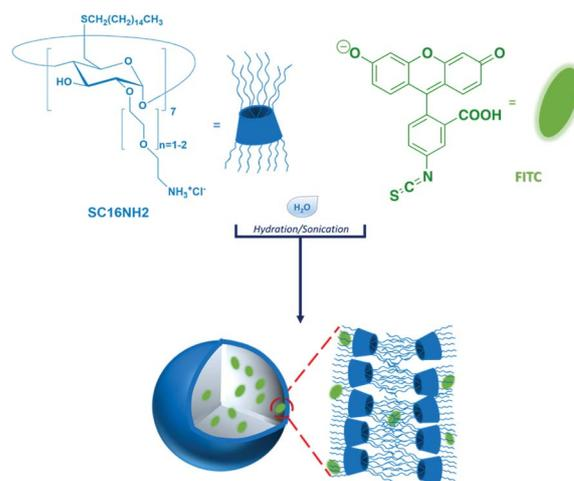
Fig. 1 Sketch of the nanosystem used in this work. Vesicles are formed by am $\beta$ CD structured in a bilayer and incorporating the FITC dye.
