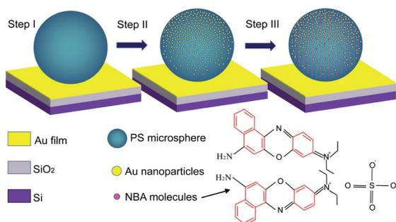
Fig. 1 Schematic of the preparation process of the photonic–plasmonic hybrid structure.
