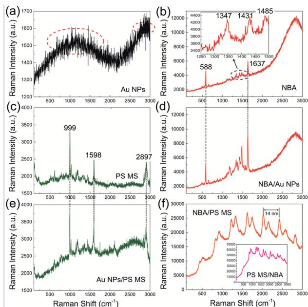
**Fig. 3** Raman spectra of (a) pure Au NPs, (b) pure NBA molecules, (c) a pure PS MS, (d) NBA molecules placed on the top surface of Au NPs, (e) Au NPs placed on the top surface of a PS MS, and (f) NBA molecules placed on the top surface of a PS MS. The inset in (b) is the zoomed spectrum in the range of 1250–1500  $\text{cm}^{-1}$ . The inset in (f) is the Raman spectrum of NBA molecules placed on the bottom surface of a PS MS.
