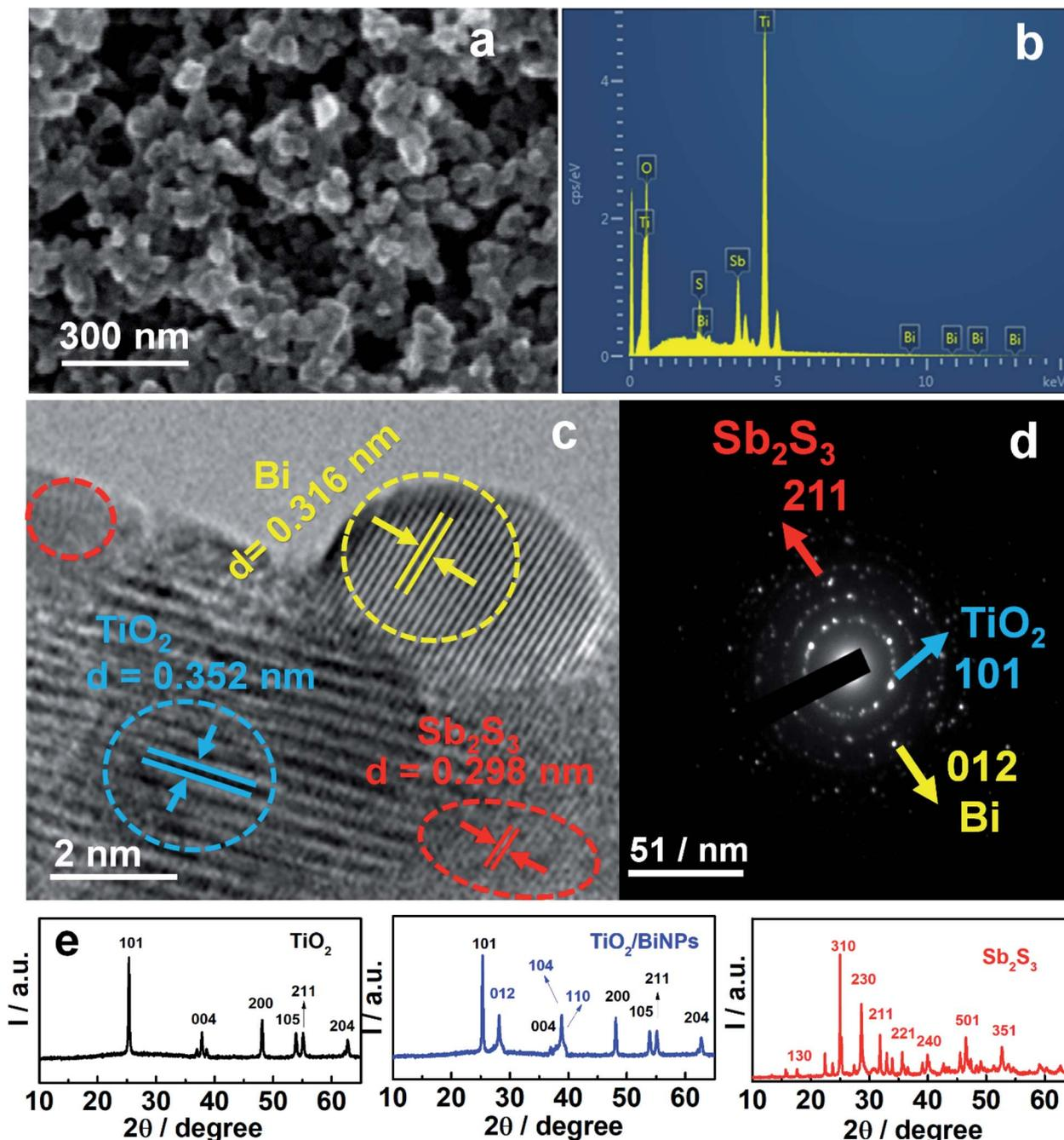
Fig. 1 Characterization of the ternary photoanode and anode materials. (a) FESEM image, (b) EDAX image, (c) HR-TEM image and (d) SAED pattern of  $\text{TiO}_2/\text{BiNP}/\text{Sb}_2\text{S}_3$ , and (e) XRD patterns of  $\text{TiO}_2$ ,  $\text{TiO}_2/\text{BiNP}$  and  $\text{Sb}_2\text{S}_3$ .
