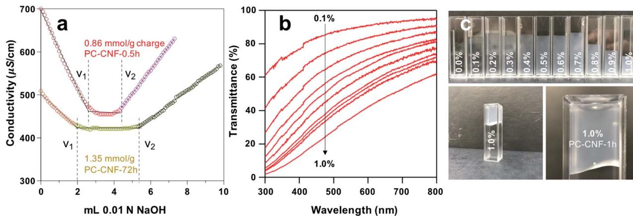
Fig. 3 Characteristics of aqueous PC-CNFs: (a) conductometric titration with NaOH (0.01 N); (b) UV/Vis transmittance of PC-CNF-1 h dispersions; (c) presence of aq. PC-CNF-1 h at increasing concentrations.
