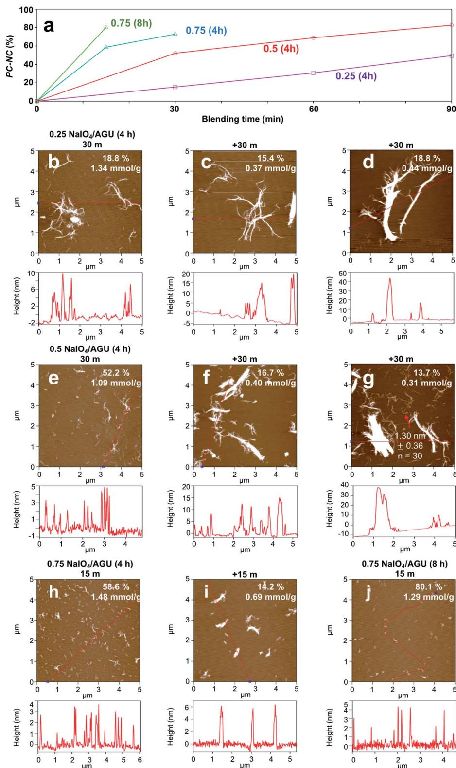
**Fig. 1** Primary periodate oxidation at varied NaIO<sub>4</sub>/AGU ratios (55 °C) and initial and additional blending time (37.5k rpm) on aqueous dispersible periodate–chlorite oxidized nanocellulose (PC-NC): (a) yield; AFM phase images and the corresponding height profiles of PC-NCs under the following conditions: (b–d) 0.25 : 1 (4 h); (e–g) 0.5 : 1 (4 h); (h and i) 0.75 : 1 (4 h); (j) 0.75 : 1 (8 h). The yield and carboxyl values of each population were noted.
