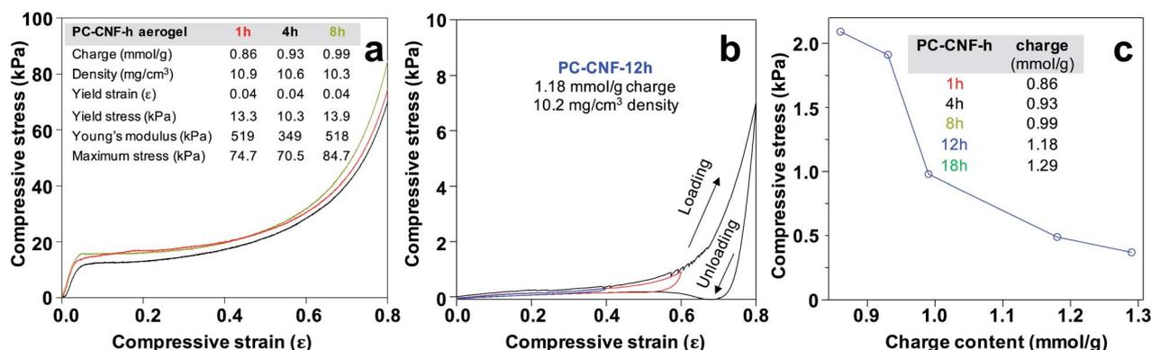
Fig. 7 Uniaxial compression of PC-CNF aerogels (1.0%): (a) dry stress–strain curves up to 0.8 strain; (b) consecutive wet compression of PC-CNF-12 h ( $1.18 \text{ mmol g}^{-1}$ ) at increasing strains of 0.4, 0.6, and 0.8; (c) ultimate wet stress at 0.4 strain of aerogels from PC-CNFs of increasing charge.
