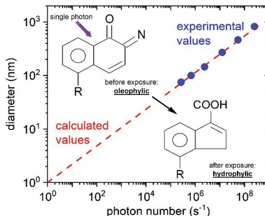
Fig. 5 For the sake of comparison our experimental data (blue circles) obtained by the LEDALIT technique are compared with theoretical values<sup>48</sup> (red dashed line) for a calculated "hole" diameter dependence as a function of photon number incident on the photoresist DNQ-sulfonate molecule. Inset: after the single photon interacts with the resist, a water-soluble carboxylic acid is formed.
