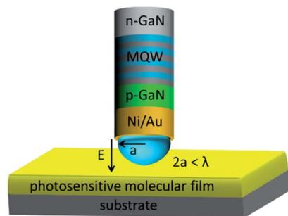
Fig. 1 Principal schematics: nano-LED (n-GaN/MQW/p-GaN) element in the near-field regime to a photochemically sensitive film generating an evanescent field. The fundamental goal of “near-field” LED assisted lithography (LEDALIT) is to create a sub-diffraction limited field distribution in a location favourable for a photochemical reaction.
