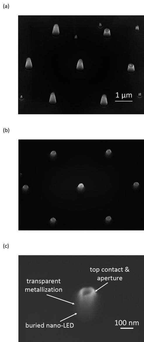
Fig. 3 Nano-LEDs after Ar-IIBE etching (a) and after covering them with a SiO<sub>2</sub> layer (b), detail of buried nano-LED structure with an aperture (c). The nano-LEDs were positioned equidistantly to each other in hexagonal arrangement with a pitch of 3 μm.
