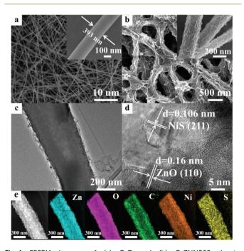
Fig. 1 FESEM images of (a) C-Z and (b) C-ZNNS60. Insets: Corresponding enlarged images. (c) TEM and (d) HRTEM images of C-ZNNS60. (e) EDX elemental mapping of C-ZNNS60.
