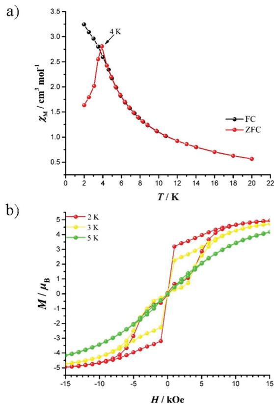
Fig. 4 (a) FC (black) and ZFC (red) magnetization plots for **8**. (b) Magnetic hysteresis loops for **8** between 2 K and 5 K with a field sweeping rate of 12 Oe s<sup>-1</sup>.
