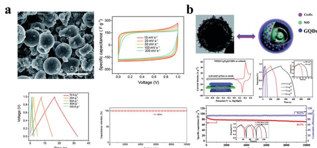
**Fig. 6** GQDs as supercapacitor additives. (a) GQDs as a conductive agent added to ultra-high specific surface area activated carbon SCs. (Reproduced with permission from ref. 77, copyright 2019 the Royal Society of Chemistry.) (b) GQDs as a conductive agent added to transition metal oxide pseudocapacitive SCs. (Reproduced with permission from ref. 78, copyright 2019 the Royal Society of Chemistry.)
