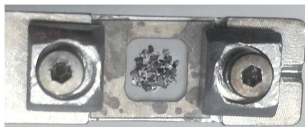
Fig. 2 A photograph of the mosaic of CrSe 2 single crystals affixed to a sapphire plate (Crystal GmbH, Berlin) using Apiezon-L grease (M & I Materials, Manchester). The tight packing and highly focused 8 Li + beam spot used in the experiment minimizes the β-NMR signal from the surrounding materials.
