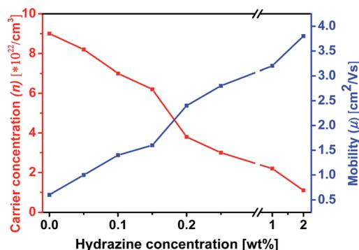
Fig. 9 Variation of carrier concentration ( $n$ ) and mobility ( $\mu$ ) of formic acid-hydrazine-treated PEDOT:PSS films with different weight concentration of proportional to hydrazine. The  $\sigma$  is proportional to  $n \times \mu$  and the  $S$  is inversely.
