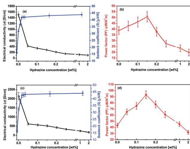
Fig. 3 TE properties of PEDOT:PSS films as a function of the hydrazine concentration. (a and b) Formic acid  $\times$  1 time and hydrazine  $\times$  1 time; (c and d) formic acid  $\times$  3 times and hydrazine  $\times$  1 time.
