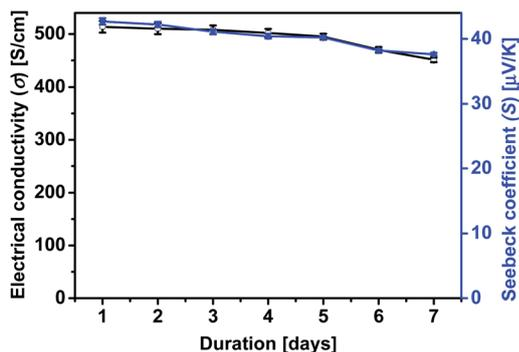
Fig. 10 The effect of stability of  $\sigma$  and  $S$  at the optimum doping level with formic acid–0.15 wt% hydrazine treatment of PEDOT:PSS film as a function of exposure time (humidity: 75%; temperature: 70 °C).
