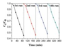
Fig. 7 Recycling runs of the spindle-like  ${\rm BiVO_4}$  for photocatalytic degradation of RhB.
