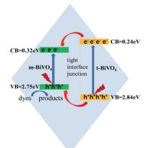
Fig. 11 Illustration of probable charge transfer on the interface junction of m-BiVO $_4$  and t-BiVO $_4$ .
