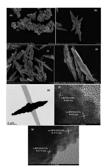
Fig. 2 SEM images of HB (a) and MB-2 (b), MB-2 (c), MB-4 (d), TEM image of MB-4 (e) and HRTEM images of MB-4 (f and g).
