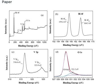
Fig. 3 XPS survey spectra of MB-4 (a) and high-resolution XPS spectra of Bi 4f (b), V 2p (c), O 1s (d).
