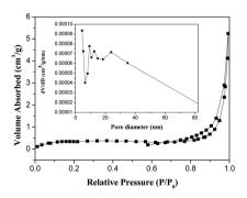
**Fig. 4** Nitrogen adsorption–desorption isotherm and pore size distribution plot of MB-4.
