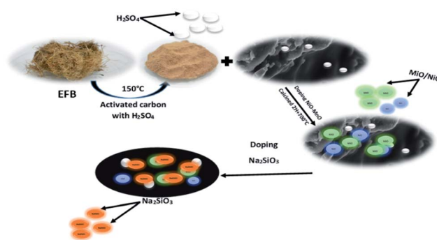
Fig. 1 Synthesis procedure of the magnetic catalysts.
