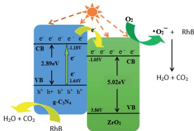
Fig. 9 Catalytic mechanism diagram of CN/ZrO<sub>2</sub> composites.
