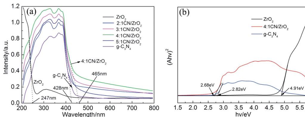
Fig. 6 UV-vis spectra of CN/ZrO<sub>2</sub> composites and pure g-C<sub>3</sub>N<sub>4</sub>, ZrO<sub>2</sub> (a); the transformed diffuse reflectance spectra (b).
