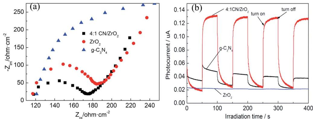
Fig. 5 EIS changes (a) and transient photocurrent responses (b) of 4 : 1 CN/ZrO<sub>2</sub> and pure g-C<sub>3</sub>N<sub>4</sub>, ZrO<sub>2</sub> electrodes.
