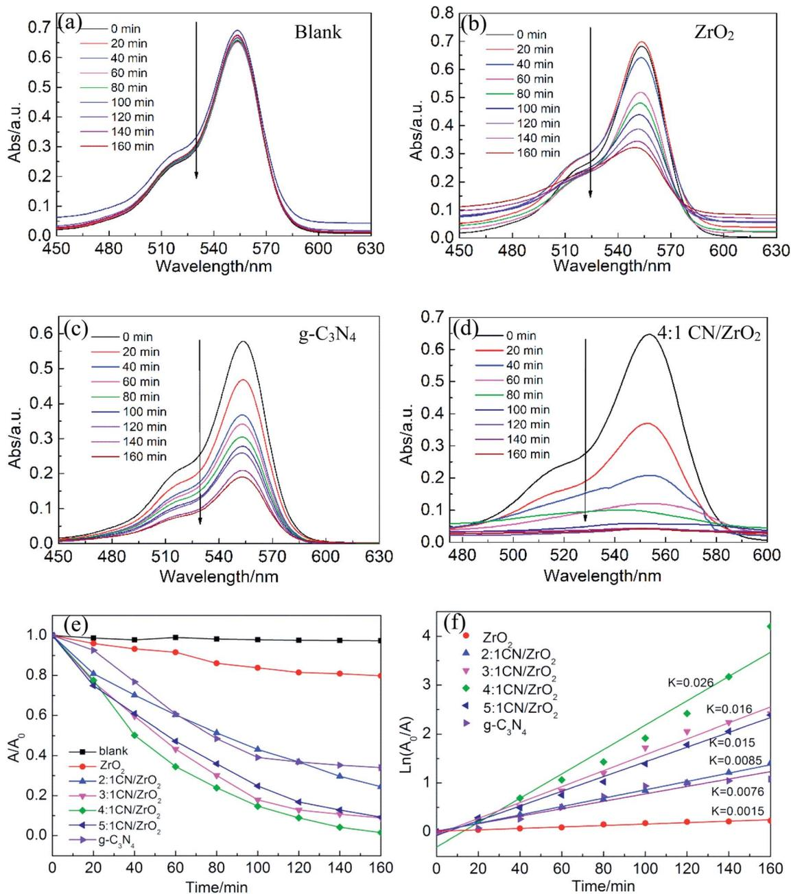
Fig. 7 UV-vis absorption spectra of photocatalytic RhB degradation over (a) blank, (b) ZrO<sub>2</sub>, (c) g-C<sub>3</sub>N<sub>4</sub> and (d) CN/ZrO<sub>2</sub> under the light irradiation. (e) Photodegradation efficiency toward RhB measured at 554 nm and (f) the photocatalytic rate curves and corresponding fitted kinetics curves of the blank experiment, ZrO<sub>2</sub>, g-C<sub>3</sub>N<sub>4</sub>, and CN/ZrO<sub>2</sub> composites under the light irradiation.
