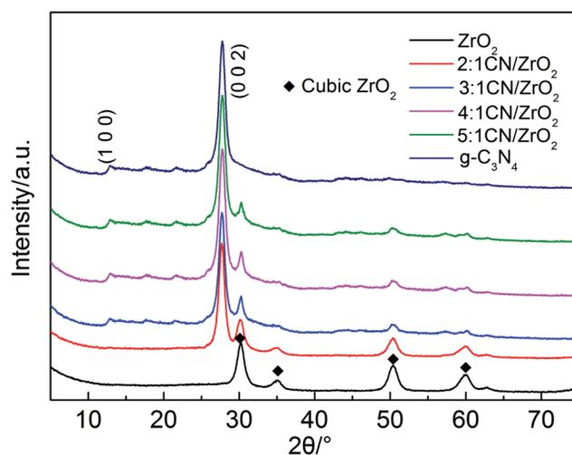
Fig. 1 XRD patterns of CN/ZrO<sub>2</sub> composites and pure g-C<sub>3</sub>N<sub>4</sub> and ZrO<sub>2</sub>.
