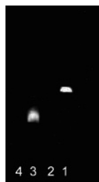
Fig. 3 Agarose gel fluorescent spectra of CdTe : Zn/ZnS QDs before and after conjugating with antibody. Note: lane 1-CdTe : Zn/ZnS QDs; lane 2-antibody; lane 3-CdTe : Zn/ZnS QDs-antibody, lane 4-PBS.
