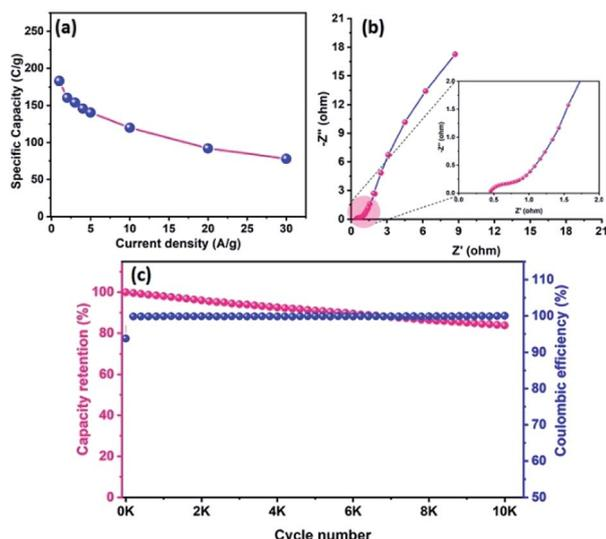
**Fig. 9** (a) Specific capacity curve of fabricated ACS as a function of different current densities, (b) Nyquist plot of CoTe NRs||OPAA ASC with the magnified view (inset), and (c) the capacity retention and coulombic efficiency of fabricated ACS as a function of cycle numbers.
