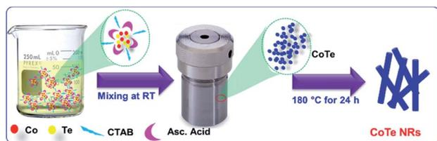
Scheme 1 Schematic representation for the growth of CoTe nanorods.
