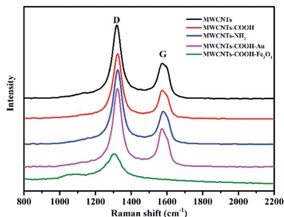
Fig. 5 Raman spectra of different MWCNTs.
