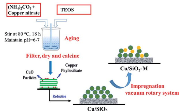
Fig. 1 Preparation process of Cu/SiO 2 -xM catalysts.
