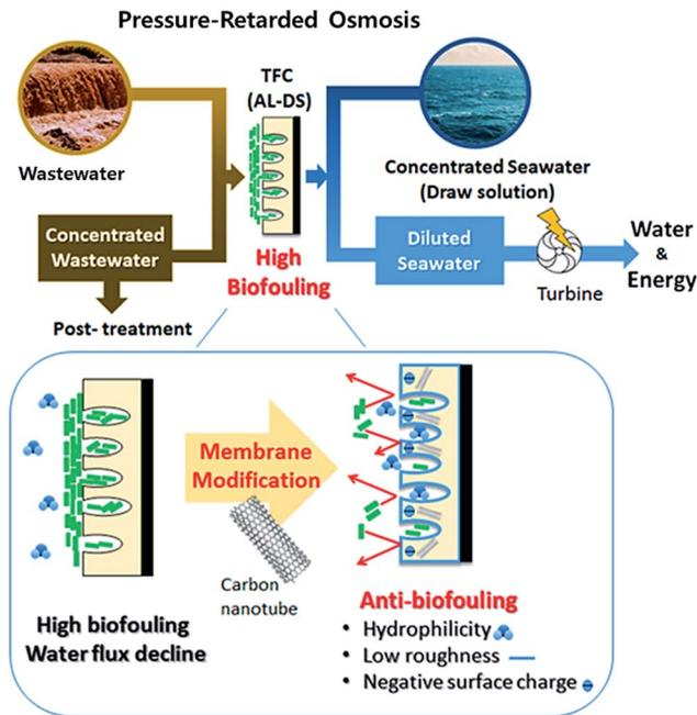
Fig. 1 Anti-biofouling properties of the TFN membrane with fCNT blended in the support layer for the PRO process.
