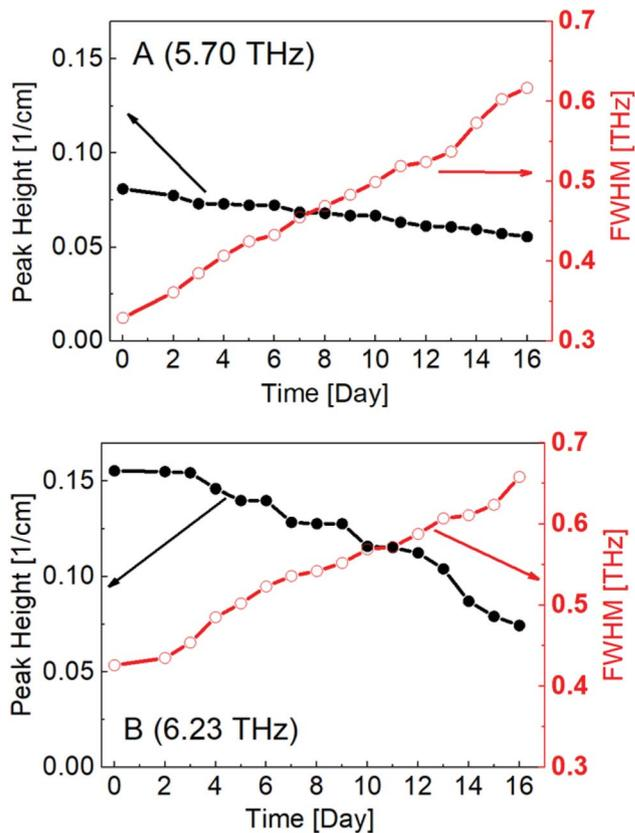
Fig. 7 Calculated peak height and FWHM values of peak A (a) and peak B (b) plotted against degradation time.
