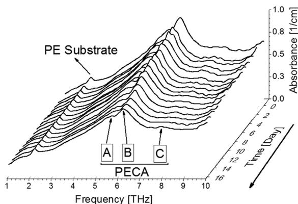
Fig. 4 THz absorption spectra of PECA degraded for different numbers of days.
