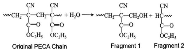
Fig. 5 Depolymerisation reaction of PECA.<sup>16</sup>
