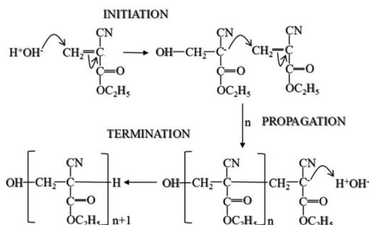
Fig. 2 Curing mechanism of 2-ethylcyanoacrylate (ECA).<sup>14</sup>
