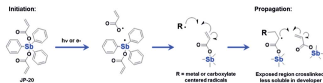
Fig. 19 A possible mechanism of polymerization of Sb organometallic compounds under illumination. Reprint with permission from ref. 36. Copyright 2015 SIPE.
