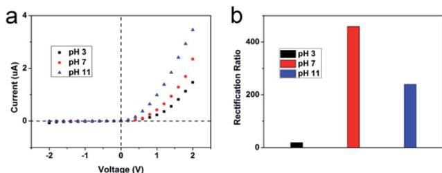
Fig. 3 Characterization of the ionic rectification in a 10 mM KCl solution at different pH values. (a)  $I$ - $V$  curves of the AAO-PVA/ $\text{WO}_3$  nanochannels measured at pH 3, pH 7, and pH 11. (b) Histogram of the rectification ratios calculated from the  $I$ - $V$  curves.
