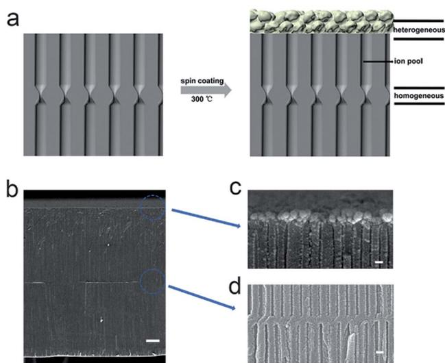
**Scheme 1** (a) A flow chart of the facile fabrication of AAO-PVA/WO<sub>3</sub> nanochannels. The nanoparticles aggregate onto the channel surfaces represent the nanoporous PVA/WO<sub>3</sub> surface coating. (b) SEM image of a cross-section of the as-prepared PVA/WO<sub>3</sub>-AAO, the scale bar is 10 μm. (c) SEM image of the surface heterojunction, the scale bar is 100 nm. (d) SEM image of the middle homogeneous junction of the hourglass-shaped AAO, the scale bar is 100 nm.
