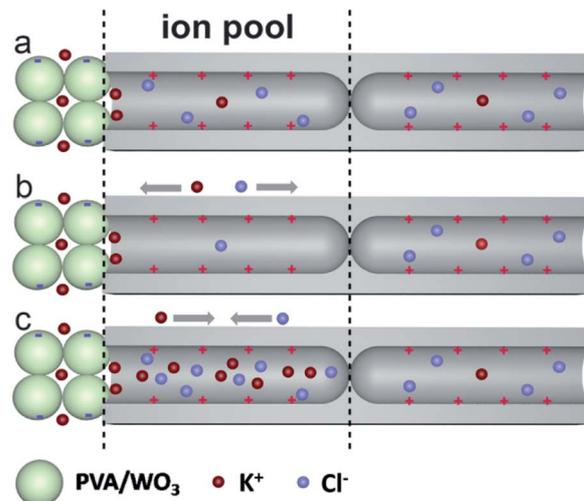
Scheme 2 Mechanism diagram of the rectifying effect under neutral condition of the PVA/WO<sub>3</sub> covered hourglass-shaped AAO. The “ion pool” is between the dashed line. (a) The equilibrium states. (b) Ion depletion state: when a negative bias is applied, both K<sup>+</sup> and Cl<sup>-</sup> would migrate to the external solution. (c) Ion enrichment state, when a positive bias is applied, both K<sup>+</sup> and Cl<sup>-</sup> would migrate to the “ion pool” area.
