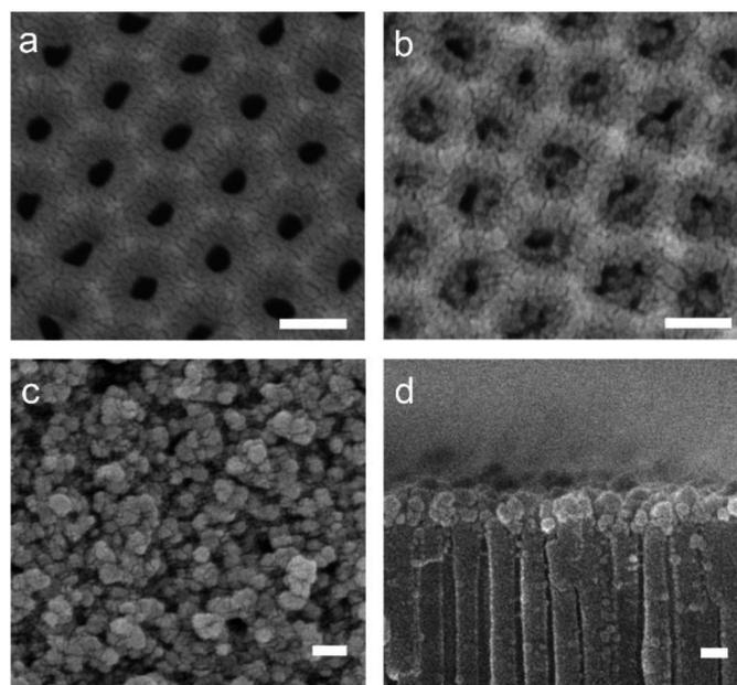
**Fig. 1** SEM images. (a) Surface of the AAO nanochannels. (b) Surface of the PVA-modified AAO nanochannels. The opening of the nanochannels were slightly blocked. (c) Surface of the PVA/WO<sub>3</sub> covered AAO nanochannels, showing that nanoporous structures were formed. (d) A cross-section of the PVA/WO<sub>3</sub> coating, showing that the opening of the nanochannels are covered with WO<sub>3</sub> nanoparticles immobilized by oxidized PVA. The scale bar is 100 nm.
