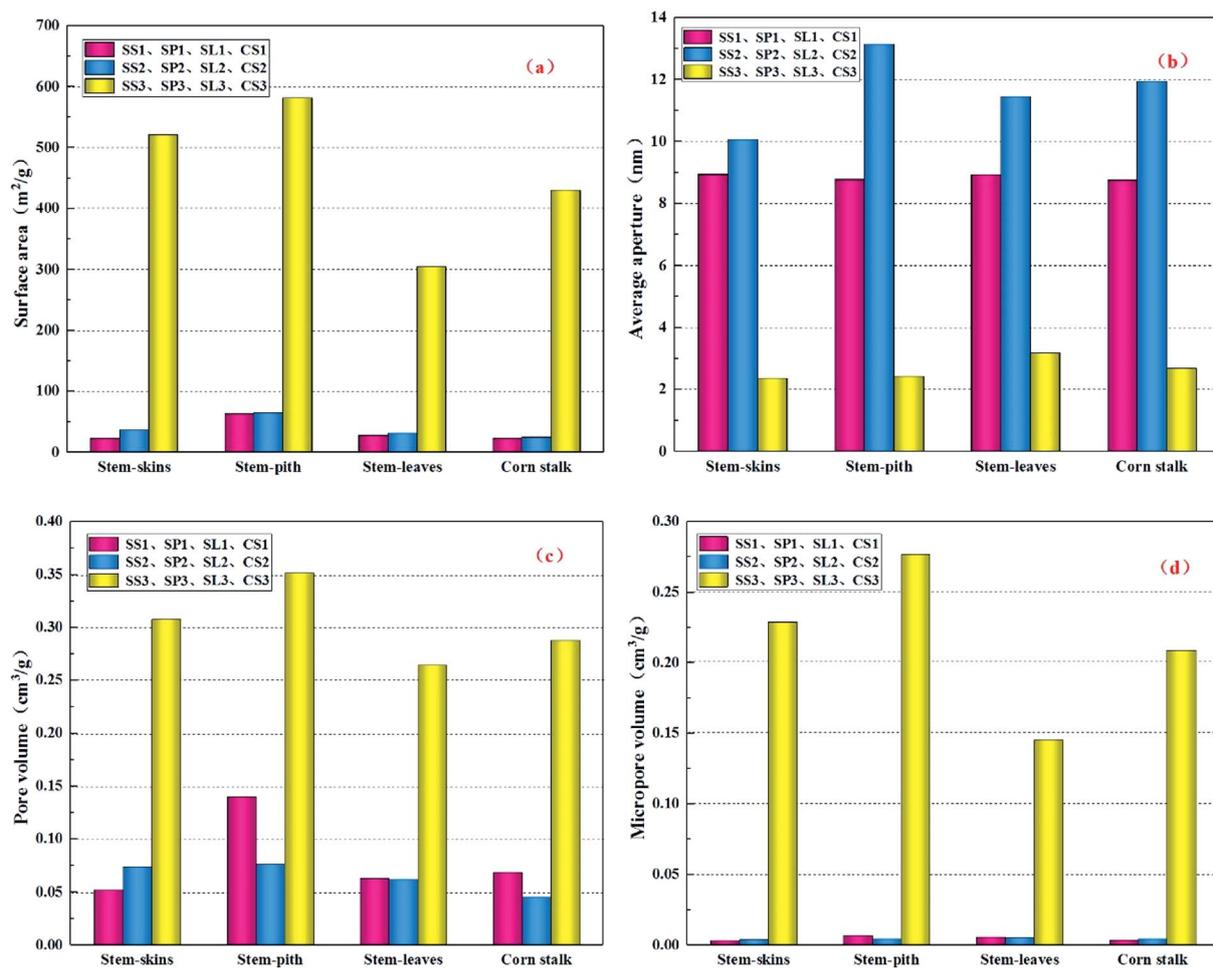
Fig. 4 Structural properties (surface area (a), pore diameter (b), pore volume (c), micropore volume (d)) of different corn stalks biochar.
