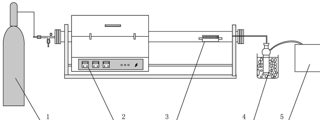
Fig. 1 Schematic draw of the experimental set-up used for pyrolysis. (1) Nitrogen (2) slide tube furnace (3) perforated quartz boat (4) pyrolysis oil collection (5) gas bag.
