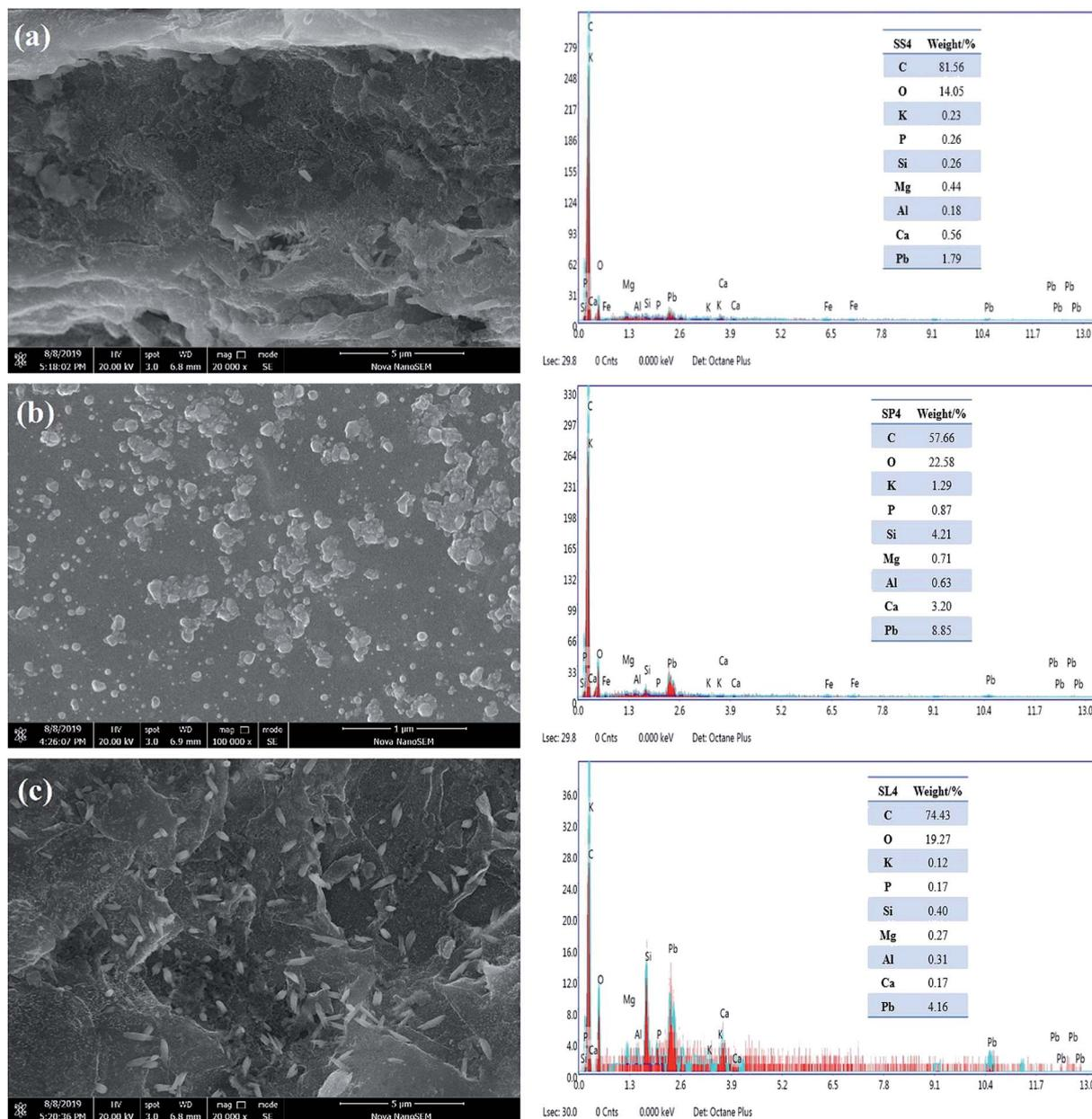
Fig. 13 SEM-EDS spectrums of stem-skins biochar (a), stem-pith biochar (b), stem-leaves biochar (c) after adsorption of Pb(II).
