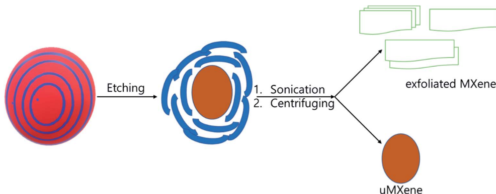
Scheme 2 The exfoliated MXene synthesis from MAX phase.
