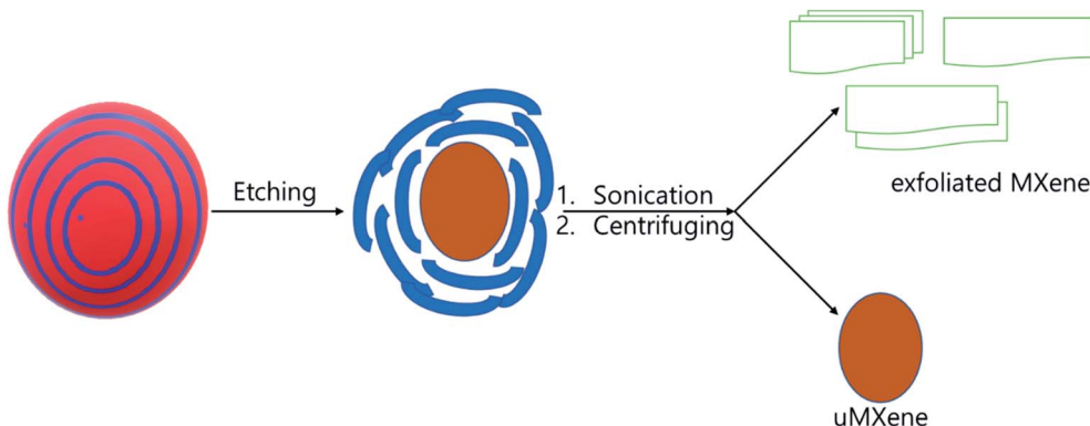
Scheme 2 The exfoliated MXene synthesis from MAX phase.
