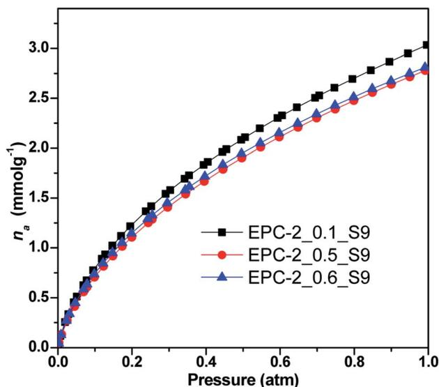
Fig. 7 CO<sub>2</sub> adsorption isotherms of EPC-2\_0.1\_S9, EPC-2\_0.5\_S9 and EPC-2\_0.6\_S9 at 273 K under pressure up to 1 atm.
