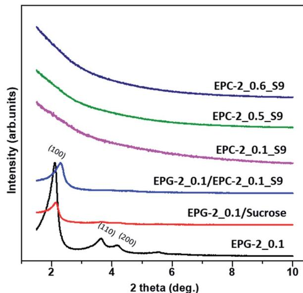
Fig. 4 X-ray diffraction patterns of (bottom to top) EPG-2\_0.1 template, EPG-2\_0.1/sucrose composite (after sucrose infiltration), EPG-2\_0.1/EPC-2\_0.1\_S9 composite (after carbonization), and replica carbons EPC-2\_0.1\_S9, EPC-2\_0.5\_S9 and EPC-2\_0.6\_S9.
