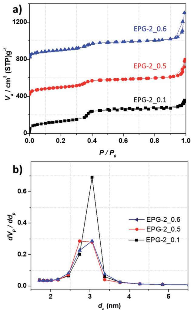
Fig. 2 (a)  $\text{N}_2$  adsorption/desorption isotherms and (b) BJH pore size distributions of EPG-2\_0.1, EPG-2\_0.5 and EPG-2\_0.6 synthesized with molar ratios of CTAB/(Si + Al) = 0.1, 0.5 and 0.6, respectively. The  $\text{N}_2$  adsorption/desorption isotherms of EPG-2\_0.5 and EPG-2\_0.6 are offset along the vertical axis by 400 and 800  $\text{cm}^3 \text{g}^{-1}$ , respectively, for clarity.
