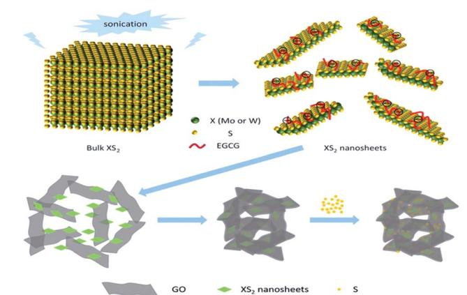
Fig. 9 Proposed adsorption mechanism of polysulfides for XS<sub>2</sub> (Mo or W).<sup>36</sup>
