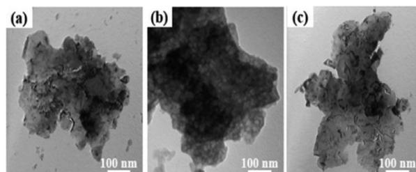
Fig. 4 TEM images of the Ni–Al alloys: (a) NAV; (b) NAA; (c) NAH.
