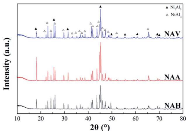
Fig. 2 XRD patterns of the Ni–Al alloys.
