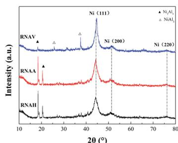
Fig. 15 XRD diagrams of the samples after hydrogenation.
