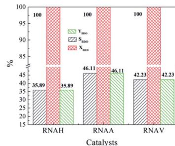
Fig. 12 Catalytic properties of RANEY®-Ni catalysts for the hydrogenation of 1,4-butenediol. Reaction conditions: 5.0 MPa (pure  $\text{H}_2$ ), 393 K, 0.5 g catalyst, 30 mL 1,4-butenediol (35 wt% in water).
