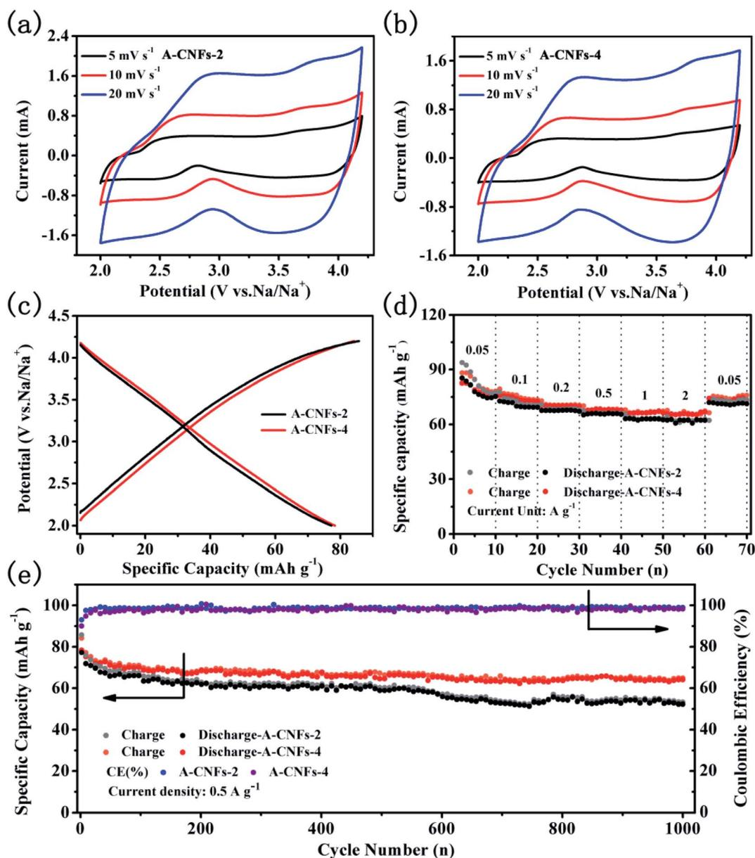
Fig. 7 CV curves of (a) A-CNFs-2 and (b) A-CNFs-4 at various scan rates in the range of 5 to 20 mV s<sup>-1</sup> in the potential range of 2–4.2 V; (c) voltage profiles of A-CNFs for the 1<sup>st</sup> cycle at 50 mA g<sup>-1</sup>; (d) rate performance of A-CNFs at various current magnitudes in the range of 0.05 to 2 A g<sup>-1</sup>; (e) cycling performance of A-CNFs for 1000 cycles at 0.5 A g<sup>-1</sup>.
