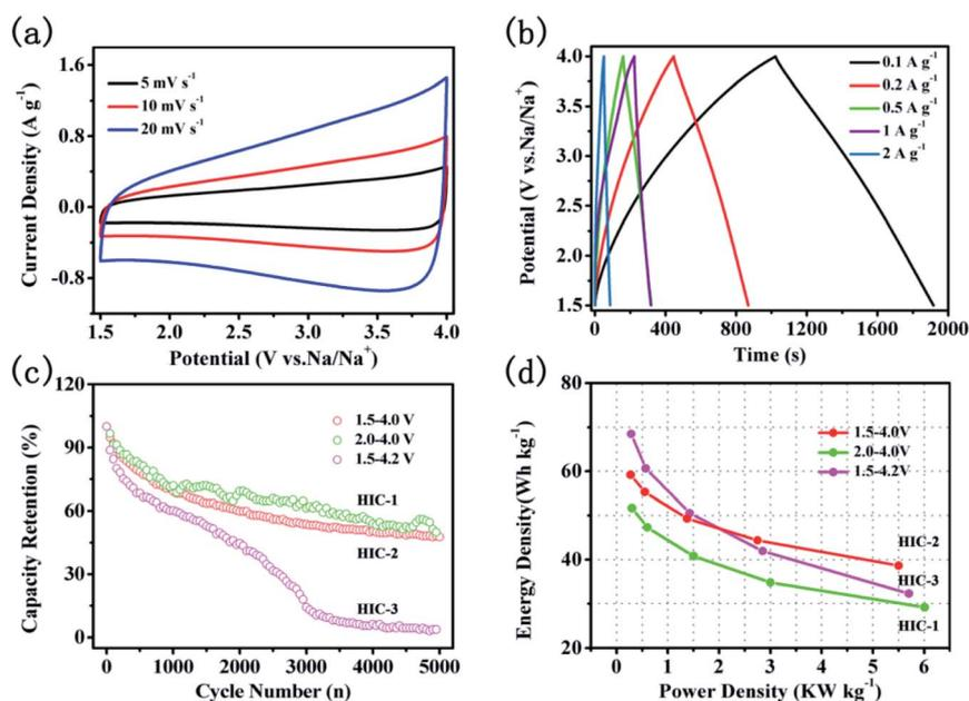
Fig. 8 Electrochemical performance of CNTs@N,O-CNFs//A-CNFs-4; (a) CV curves at various scan rates in the range of 5 to 20 mV s<sup>-1</sup> in the potential range of 2–4 V; (b) galvanostatic charge/discharge curves at various current densities from 0.1 to 2 A g<sup>-1</sup>; (c) the capacity retention over 5000 cycles at the current magnitude of 0.5 A g<sup>-1</sup>; (d) Ragone plots for various voltage ranges.
