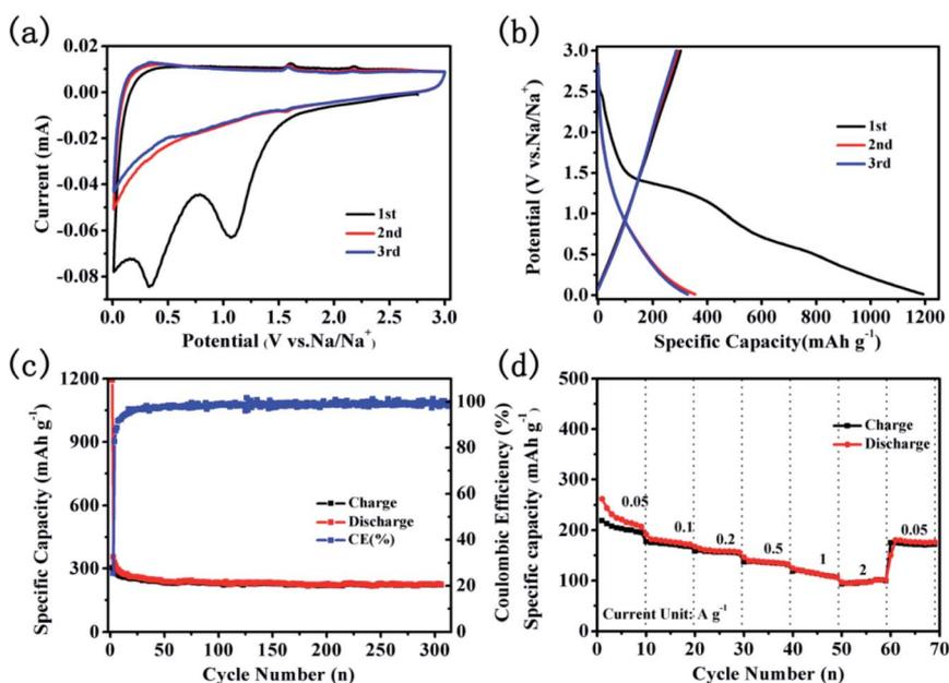
Fig. 4 Electrochemical performance of the CNTs@N,O-CNFs electrode; (a) three initial CV curves at a scan rate of 0.1 mV s<sup>-1</sup> in the potential range of 0.01–3 V; (b) voltage profiles for the 1<sup>st</sup>, 2<sup>nd</sup>, and 3<sup>rd</sup> cycles at 50 mA g<sup>-1</sup>; (c) cycling performance for 300 cycles at 50 mA g<sup>-1</sup>; (d) rate performance at various current magnitudes in the range of 0.05 to 2 A g<sup>-1</sup>.
