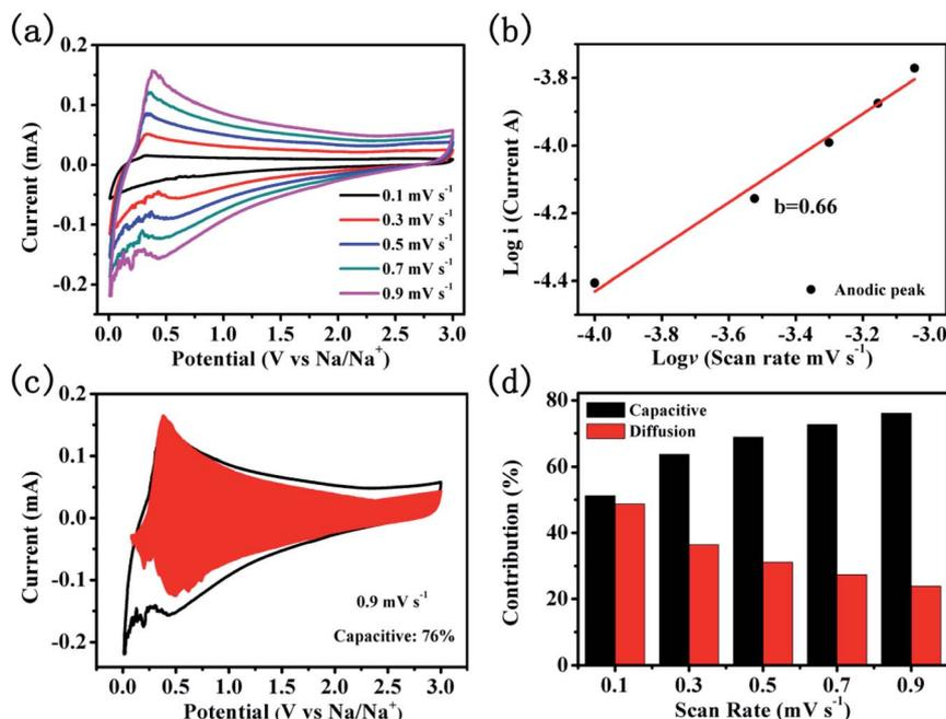
Fig. 5 Quantitative capacitive analysis of sodium storage mechanism. (a) CV curves of the CNTs@N,O-CNFs electrode at various of scan rates; (b) relationship of the cathodic peak current and the scan rates for the CNTs@N,O-CNFs electrode; (c) capacitive contribution of the CNTs@N,O-CNFs; (d) charge contributions from the diffusion/capacitive-controlled process as a function of scan rate.
