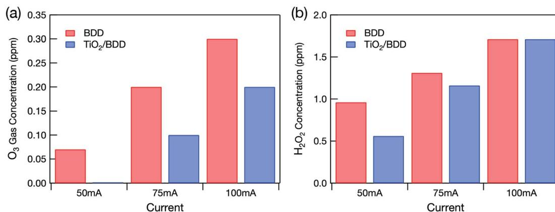
Fig. 2 Concentrations of (a) O<sub>3</sub> gas from the glass cell and (b) H<sub>2</sub>O<sub>2</sub> dissolved in treated water caused by the application of different constant currents to BDD and mesoporous TiO<sub>2</sub>/BDD hybrid electrodes.
