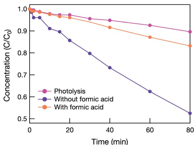
Fig. 4 Time dependence of MB concentration estimated from visible spectra during the photocatalytic (under 222 nm illumination) water treatment test of mesoporous TiO<sub>2</sub>/BDD hybrid electrode with and without 1 mM formic acid (a sacrificial reagent added to react with holes). C and C<sub>0</sub> are the remaining and initial concentrations of MB, respectively.
