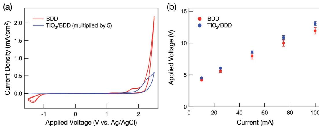
Fig. 1 (a) Typical cyclic voltammogram of BDD and mesoporous TiO<sub>2</sub>/BDD hybrid electrodes in a 0.25 M phosphate aqueous buffer solution at a scan rate of 0.1 V s<sup>-1</sup>. The current density in the hybrid electrode was multiplied by five. (b) Relationship between applied voltage and current in BDD and mesoporous TiO<sub>2</sub>/BDD hybrid electrodes in a 0.25 M phosphate aqueous buffer solution.
