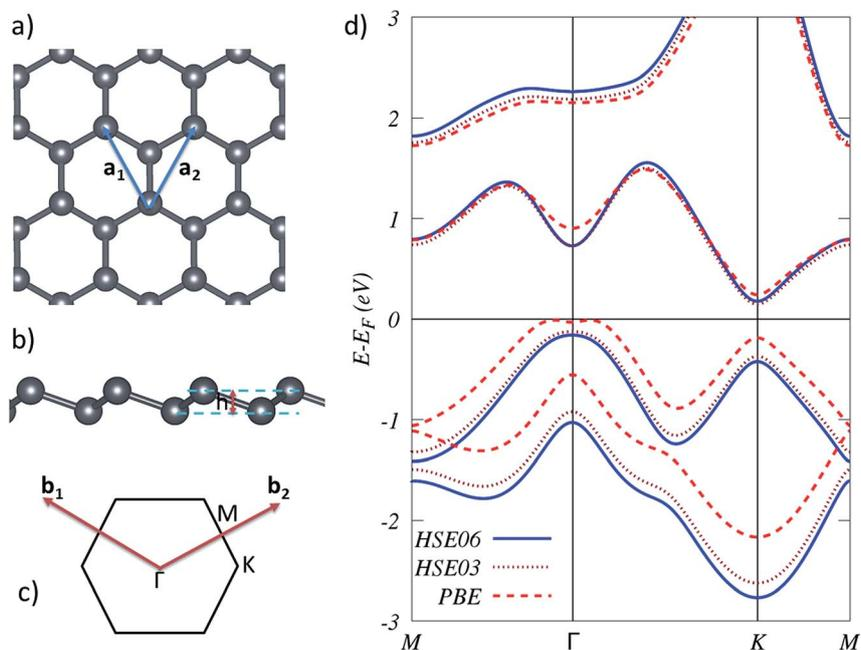
**Fig. 1** (a and b) Top and side views of buckled plumbene, respectively. The blue solid vectors indicate the primitive vectors.  $h$  is the vertical distance between the Pb planes. (c) First Brillouin zone with high-symmetry points. (d) Electronic band structures for plumbene calculated with the HSE06 (blue solid line), HSE03 (brown dotted line), and PBE (red dashed line) functionals.
