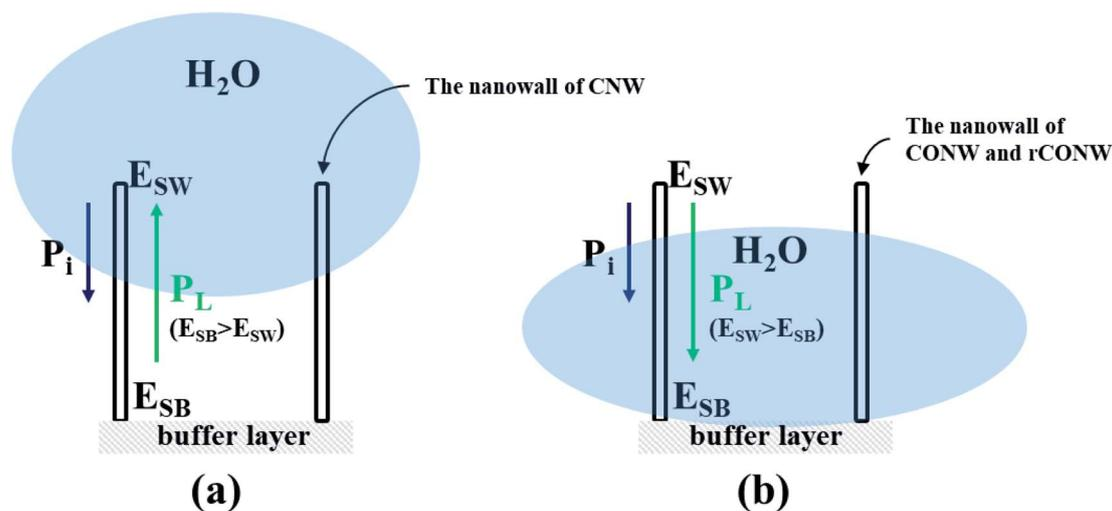
Fig. 2 Schematic of variation in contact angle according to the energy difference between the nanowalls and the surfaces in the (a) CNW and the (b) CONW and rCONW.
